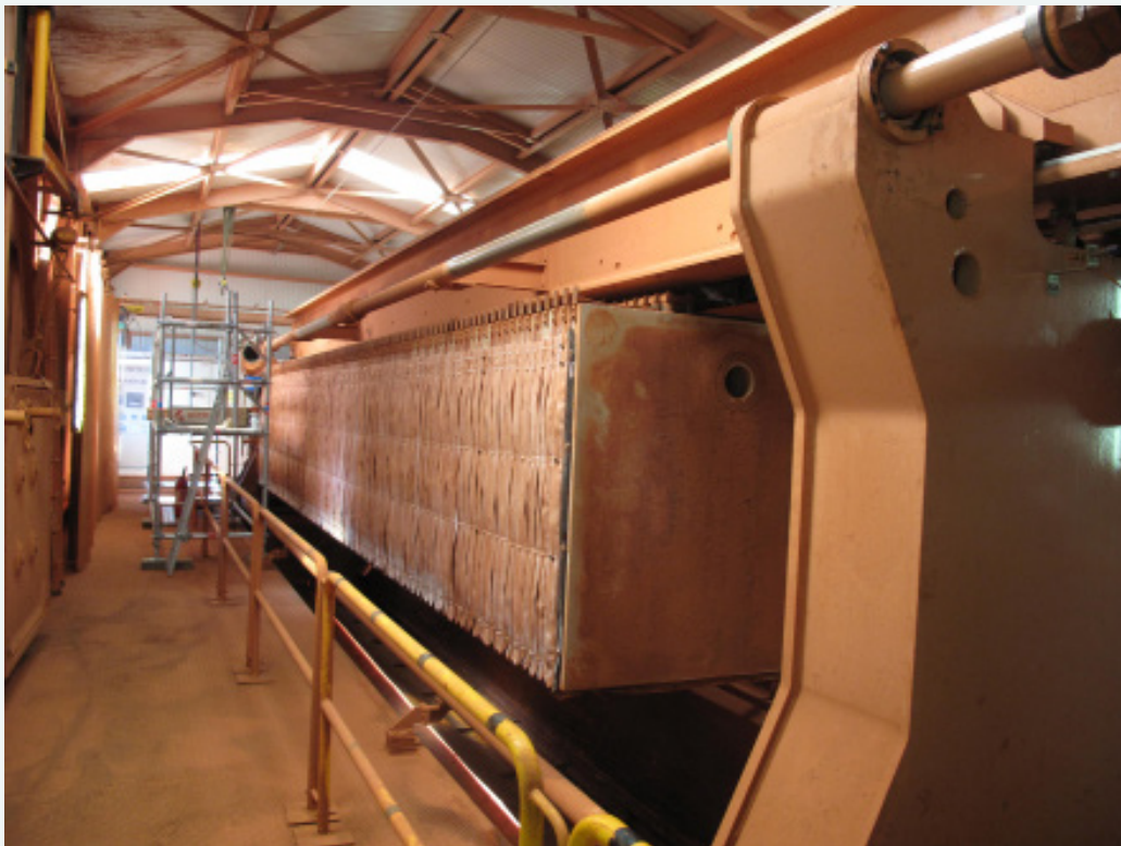
Filter press at Gardanne refinery
