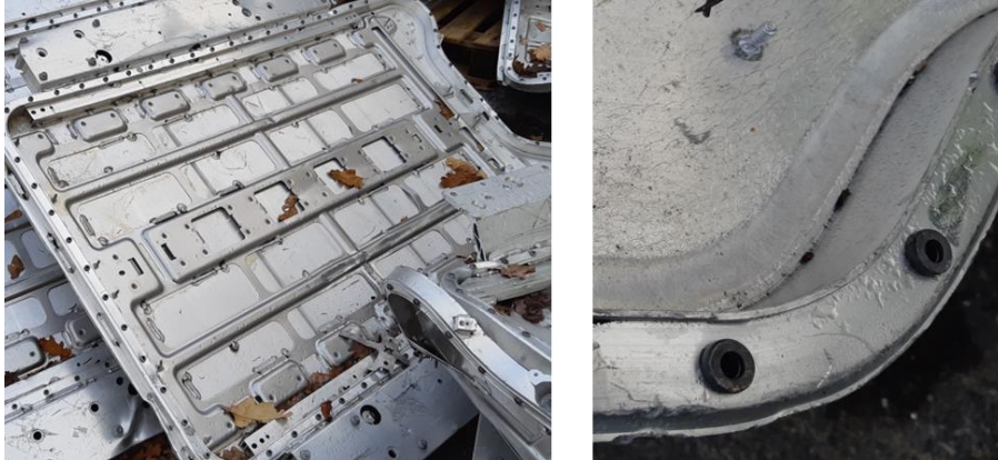
Figure 20: Example of scrap pollution in eV battery casing (steel screws) (pictures from M2P at a French refiner scrap yard)
