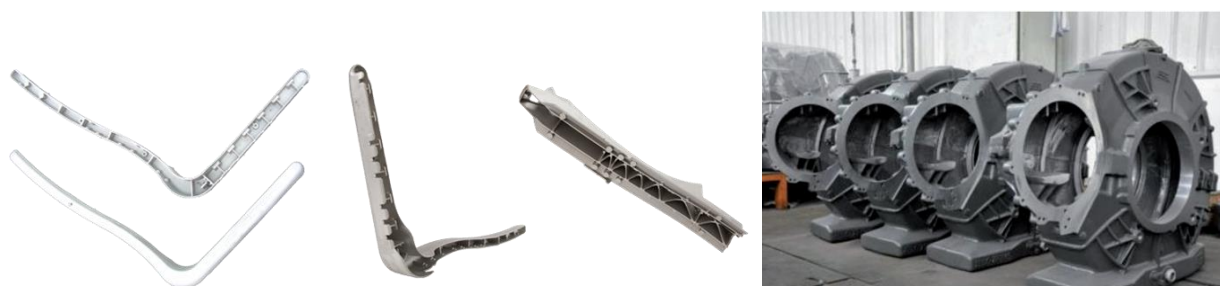
Figure 14: Railway seat frame elements AlSi7Mg0.3 (Pictures from fonderie-aluminium-declercq.fr) ; gearbox housing on the right from Sun (Sun, Han, and Dong 2021)
