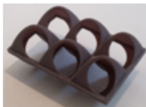
Fig 6.18 Wax prototype for the shells of the solar shading at the Nasher Sculpture Center
