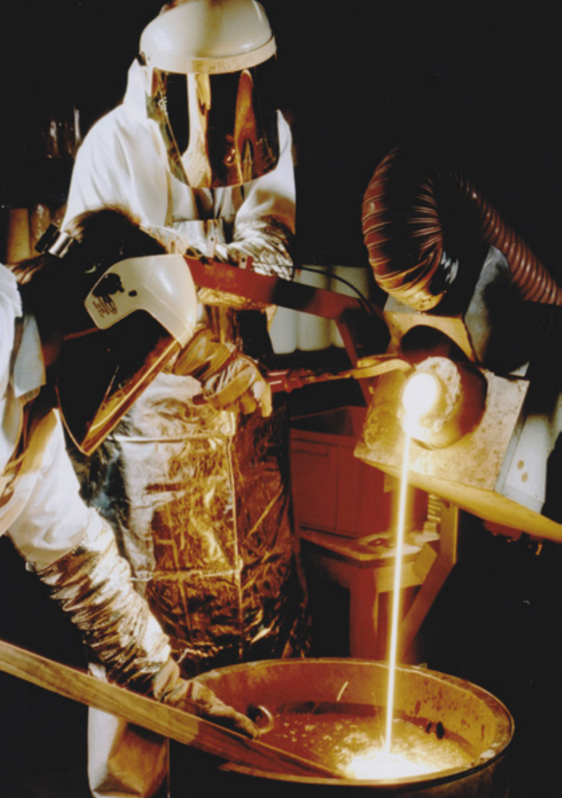
Fig. 2.40 Pouring molten recycled aluminium in a foundry
