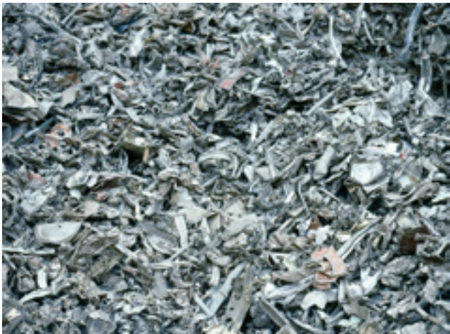
Fig 2.35 Shredded aluminium scrap
