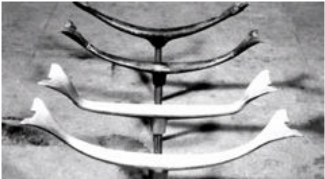
Fig 6.6 Early prototypes of the cast aluminium component of the Aluminum Group chair by Charles and Ray Eames
