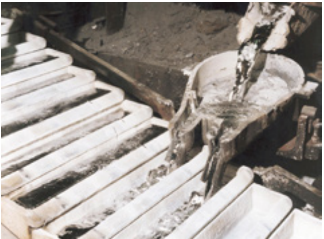
Fig 2.37 Casting recycled aluminium
