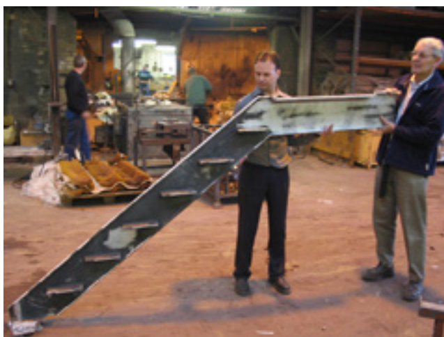
Fig 6.36 Internal face of cast aluminium stringer showing connection flanges
