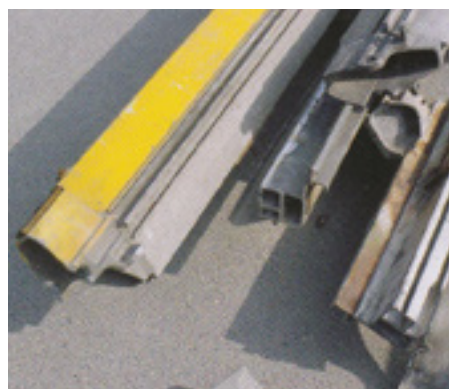
Fig. 4.44 The aluminium extrusions from the original pavilion in Paris had been cut and welded to alter the height of the pavilion in Lille
