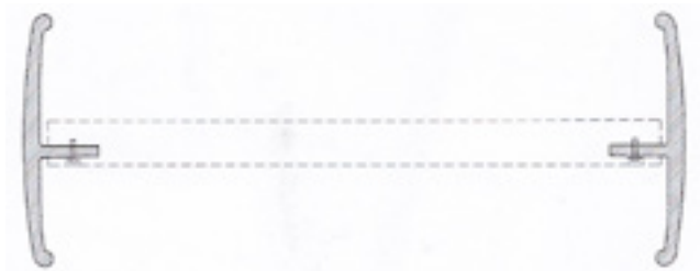
Fig 6.34 Section through a pair of stringers, showing lug plates that support the timber treads
